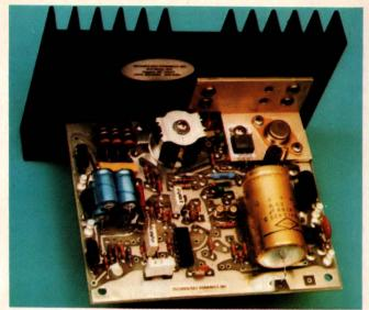
**Switching regulators,** such as Technology Dynamics' Model SR50P, can deliver 50W in a small package.
