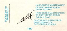
Fig 8—Very large memory systems generally experience increased reliability with relatively short hard- or soft-error maintenance intervals. For most other memory systems, though, shorter maintenance intervals can provide only a modest reliability improvement.
