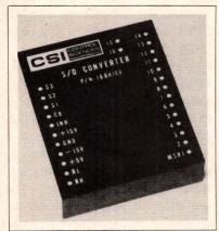
SYNCHRO CONVERTER. Employing Type II servo loops designed to follow input-shaft velocities as high as 1800°/sec (300 rpm), the 16-bit Model 168H100 synchro- or resolverto-digital unit provides 1.3' accuracy over its full temperature range. It maintains this performance despite ±10% signal- and reference-amplitude
