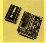
ADC 2000/2100 16-BIT A/D CONVERTERS for airborne, other critical applications. Resolution of ADC 2000/2100 series is 1 part in 65,535—16 binary bits or 2's complement; power consumption only 500 mw; accuracy: ±0.004%; linearity: ±0.002%; output control functions CMOS/TTL-LS compatible with any system. Tested, calibrated, system-ready except for power supply. ADC 2000: P.C. Card; ADC 2100: Encased. PHOENIX DATA, INC., 3384 W. Osborn, Phoenix, AZ 85017. PH 602/278-8528.
