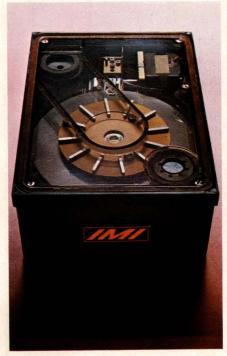
Employing a plated medium, dual impellers and temperature-compensation circuitry, the International Memories 5000 Series 5.25-in. Winchesters will initially be offered with 7M-byte unformatted capacity.
