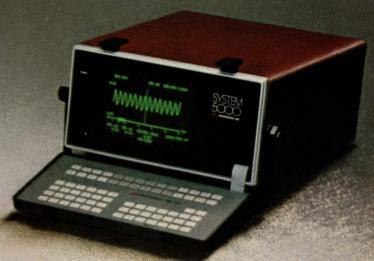
40 Channels for Hardware/Software/ Analog Waveform Analysis Model PI-540 Logic Analysis System \$9,950.
