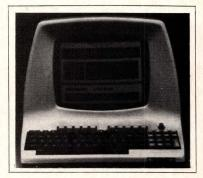
transmission of data to any serial RS-232C peripheral device. It also features a teletypewriter-style keyboard, a built-in numeric keypad, separate cursor-control keys and a full upper-and lower-case 12-in.-diagonal character display with 2-dot descenders as standard. Characters are displayed as a 5×9 dot matrix in a 7×10 dot-matrix field. A Program-mode key permits writing into the display memory as well as the display of
