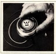
PHASE-CONTROL SCR. A phase-control thyristor that can handle up to 3500V and provide current ratings of 800 to 1200A, Model T9GO minimizes the need for series design in high-voltage circuits. Developed for motor and phase controls, VAR systems, power supplies and fusion systems, it provides guaranteed dv/dt of 300V/μsec. Forward voltage drop specs at 1.7V for the 1200A unit. Other features include gate current of 200A with soft gate control,
