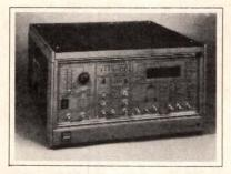
bit-error-rate measurements to 325 MHz, the modular BERTS-325C includes a clock source, transmitter and receiver that generate pseudorandom or fixed-word patterns for stimulating the system under test and measure the bit-by-bit errors received. BER or total errors can be measured on continuous or burst data for applications such as TDMA testing. Data and delayed-data outputs are furnished for QPSK-test applica-
